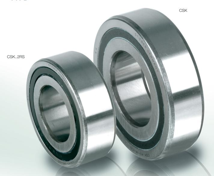
Type CSK is a sprag type freewheel integrated into a 62 series ball bearing (except sizes 8 and 40). It is bearing supported, delivered grease lubricated and protected against dust of more than 0,3 mm. The use of additional "nylos" type seals is recommended especially when the working temperature exceeds 50°C. Oil bath lubrication is also possible.
